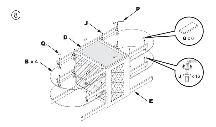
8-Fasten glass (B) to the frames (D&E) with screws (J). Fix the rubber Feet (Q) on the frame (D&E)
